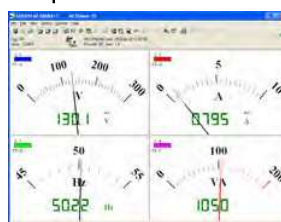
Multimeter Display for Up to 4 Channels
