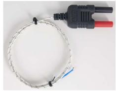
Type K thermocouple with banana plugs
