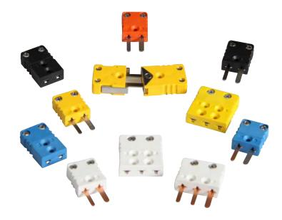
Watlow's line of miniature connectors offer a wide range of solutions for your temperature sensing needs. These miniature connectors feature a rugged glass-filled thermoplastic body, captive terminal plates that allow for faster wire termination and locking connectors. Some offer ultra-high temperature capabilities as well. Listed below are the various miniature connectors and systems from which to choose:
