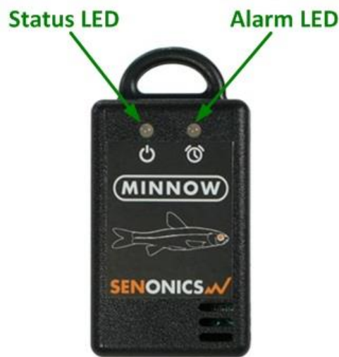
Figure 2: Minnow Alarm Indicators
