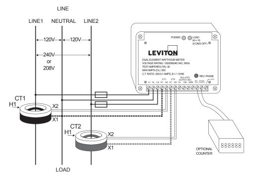
Leviton recommends solid core transformers (CTs) for revenue-grade accuracy. Our 100A and 200A color coded CTs assist with correct installation by indicating phase monitored. Split core CTs are also available upon request for applications where power cannot be interrupted during installation. Our 100-5,000 Amp Split Core CTs offer +/-1.0% accuracy.
