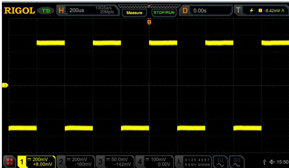
Figure 4-2 Waveforms before Averaging
