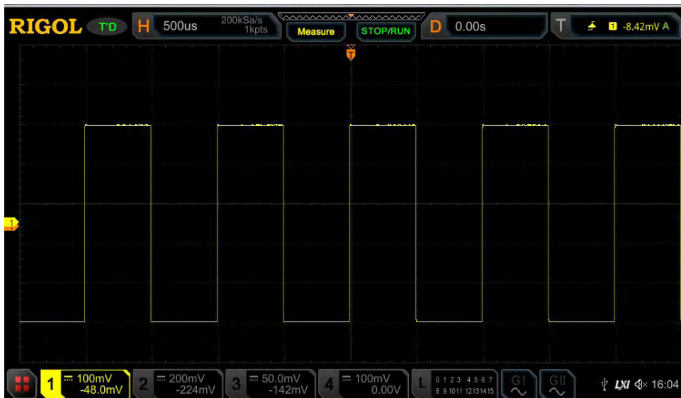
Figure 4-3 Waveforms after 128 Times of Averaging
