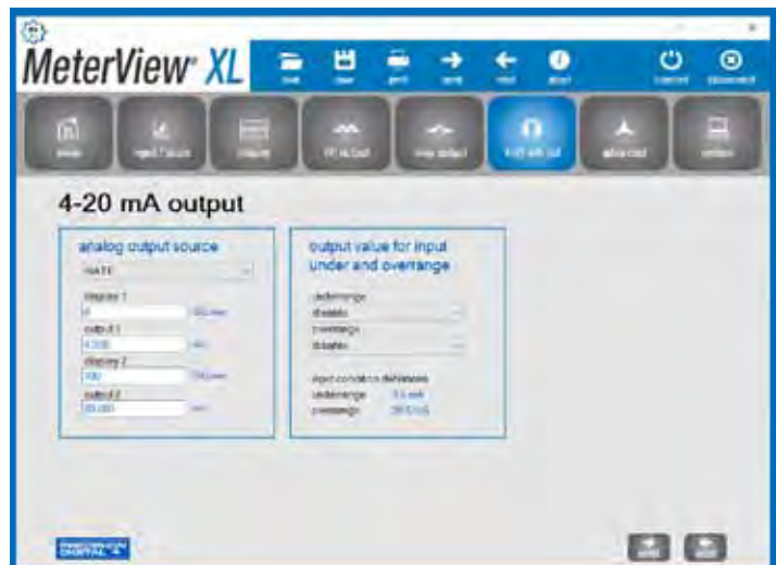
▲ The 4-20 mA Output window is used to program the isolated 4-20 mA output's source, range, and under and over range values.
