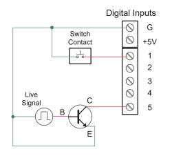
Figure 6. Digital Input from Switch Closure and Live Signal
