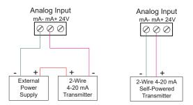
Figure 3. Transmitter Powered by External Supply or Self-Powered
