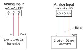
Figure 2. Transmitters Powered by ConsoliDator+'s Isolated 24 VDC Power Supply
