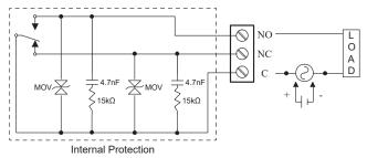
Figure 11. AC and DC Internal Inductive Load Protection
