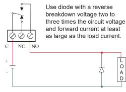
Figure 12. Low Voltage DC Loads Protection
