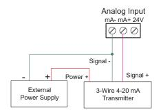
Figure 4. Three-Wire Transmitters Powered Externally
