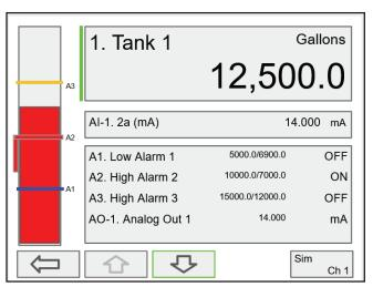
**Active High Alarm:** Indicated by horizontal and vertical lines. The bottom of the vertical line is the reset point of the high alarm. The high alarm is indicated on the left side of the bargraph.
