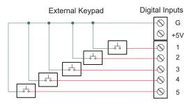
Figure 14. External Keypad Connections
