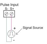
Figure 5. Flow Meter Pulse Input Connections
