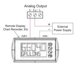
Figure 8. Passive 4-20 mA Output Powered by External Supply
