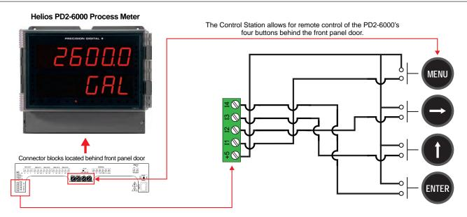
Use the PDA2364-MRUE to remotely control the PD2-6000's four internal programming and operation buttons which are located behind the door below the display.
