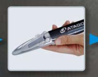
**2** Close the daylight plate. View the scale through the eyepiece.
