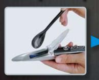
1 Apply 1-2 drops onto the prism.
