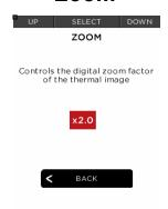
While imaging, press and hold the left button to continuously zoom up to 4X. You can also set the zoom factor manually in settings.
