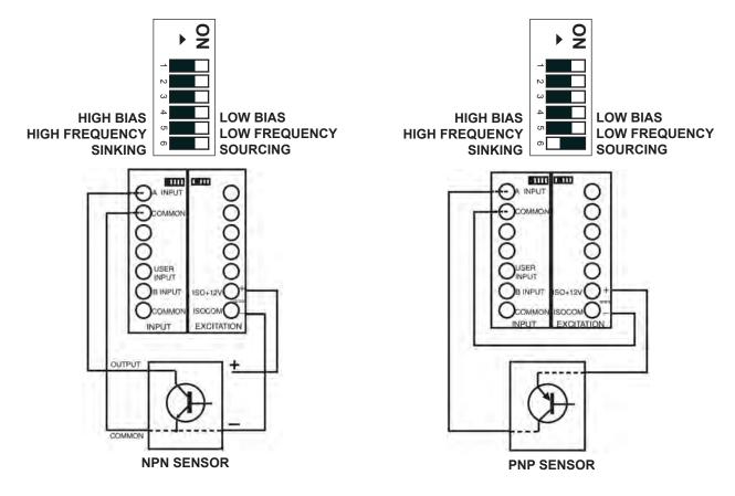
Figure 8. Sensor Connection Examples
