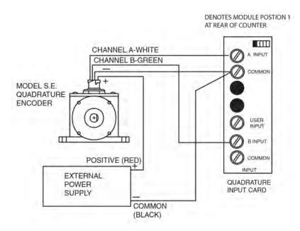
Figure 12. Wiring Encoder with External Supply
