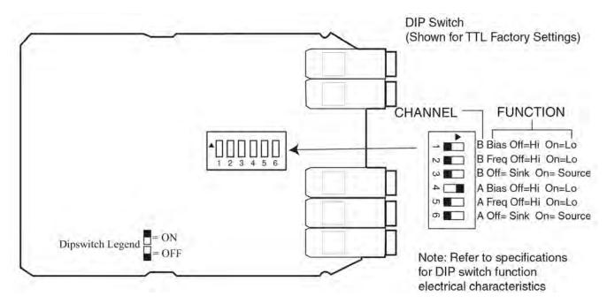
Figure 7. Standard Input Module Default Settings
