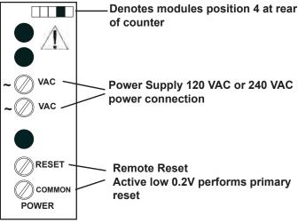
Figure 5. AC Power Module
