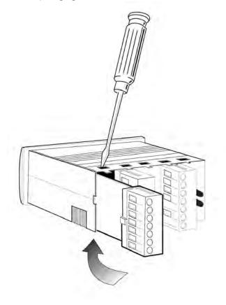
Figure 4. Removing Option Module
