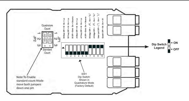
Figure 10. Quadrature Input Module Default Settings
