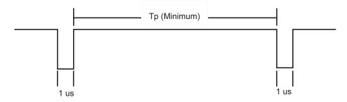
Figure 15. Input Pulse Definition
