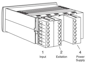
Figure 1. Option Module Slots (Rear View)
