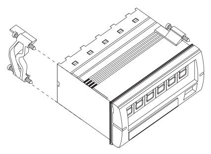
Figure 3. Panel Mounting Clips
