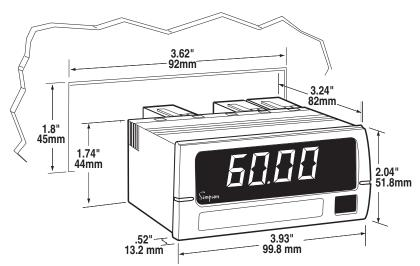
Figure 2. Counter and Panel Cut-Out Dimensions
