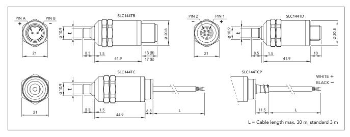
The DuoTech accelerometer is a single transducer solution used for vibration or shock pulse measurements or both in combination. The accelerometer is mounted in a countersunk mounting hole identical to holes normally used by shock pulse transducers.
