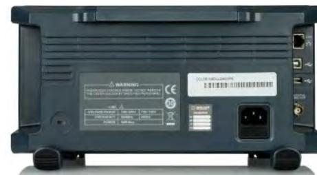
Back panel of T3DSO1104, T3DSO1202A, T3DSO1204, T3DSO1302A
