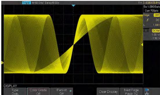
New display technology provides for fast refresh rates. The resulting intensity-graded trace is brighter for events that occur with more frequency and dims when the events occur with less frequency.
