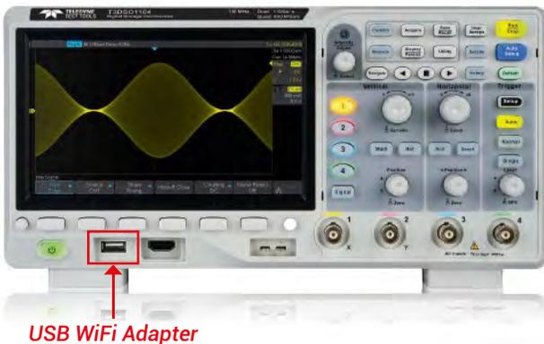
WiFi control of instrumentation can provide a convenient and safe method of configuring and collecting data. This new feature works with a Teledyne Test Tools approved WiFi adapter to provide wireless control and communications with Teledyne Test Tools 4 channel scopes. Option not available for the T3DSO1102. The approved adapter is the TP-Link TL-WN725N (not supplied).
