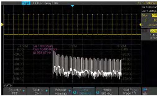
The math co-processor enables FFT analysis of incoming signals using up to 1 M samples per waveform. This provides high frequency resolution with a fast refresh rate. The FFT function also supports a variety of window functions so that it can adapt to different spectrum measurement needs.
