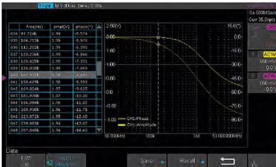
T3DSO1000 can control the USB AWG module, control an independent Teledyne Test Tools T3AFG instrument, scan an object's amplitude and phase frequency response, and display the data as a Bode Plot. It can also show the result lists, and export the data to a USB disk. Not available for the T3DSO1102.
