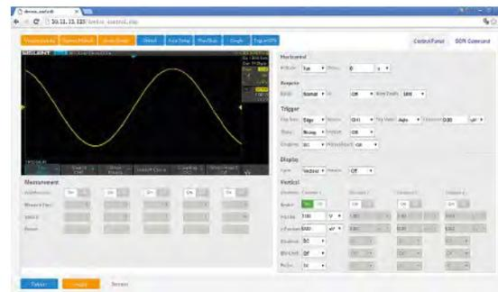
With the new embedded web server, users can control the Oscilloscopes from a simple web page. This provides remote troubleshooting and monitoring capabilities.
