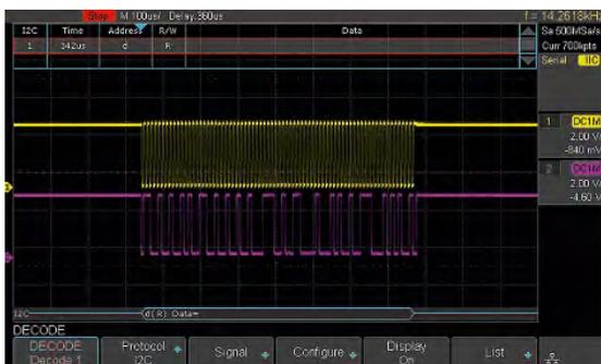
T3DSO1000 displays the decoding through the events list. Bus protocol information can be quickly and intuitively displayed in a tabular format.
