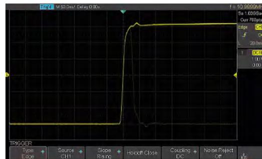
With a waveform capture rate of up to 400,000 wfms/s (sequence mode), the oscilloscope can easily capture the unusual or low-probability events.
