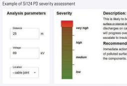
Description: This is likely to be a very strong surface or internal discharges. Surface or internal discharges on cables, terminations, and joints will progress over time and might rapidly escalate to insulation breakdown. Recommendation: Immediate action. Visual Inspection. Cleaning of polluted surfaces. Repair or replacement of
