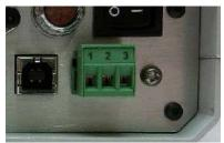
Figure 1: Relay screw-terminal header
