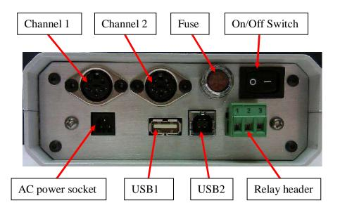
Channel 1 & 2 – Female sockets for probe connections.
