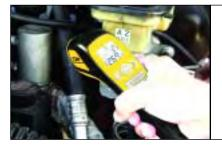
The unit offers simple one-handed operation, laser point sighting, a backlit display, °C/°F select ability and an automatic power off feature.
