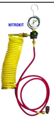
**NITROKIT** automotive Air Conditioning Nitrogen Pressure Leak Test Kit. This kit is needed to pre-check automotive A/C systems for leaks due to loose mechanical connections, leaks in hoses, evaporators and condensers, before re-introducing refrigerant back into the A/C system. This will prevent unnecessary leakage of refrigerant into the atmosphere.
