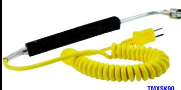
The TMXSK90 is the fastest and most accurate handheld K-type surface probe providing accurate readings in less than 5 seconds. The sensor is made from flat-spring ribbons of thermocouple material for contact on uneven surfaces. An angled head for measuring hard to reach surfaces and a 3 foot coiled lead for durability and long reach. The exposed junction provides for fast response and is compatible with any other instrument with a K-Type input.
