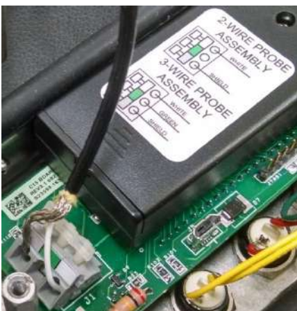
Figure 1: Probe Assembly Lead Attachment
