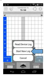
A new box will appear with three selectable time increments: hours (hh), minutes (mm), and seconds (ss). Set the desired increment (how often to record each reading) and select start.
