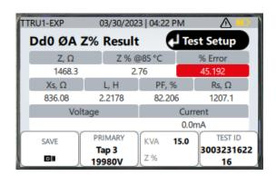
Click and hold the enter button for three seconds to view additional test information, including measured impedance, reactance, inductance, power factor, and AC resistance, and test voltage and current.
