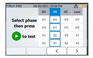
When testing three phase vectors, using the enter button to return to the test setup and then pressing play will highlight the next phase to be tested, guiding the customer through all three phases of tests.
