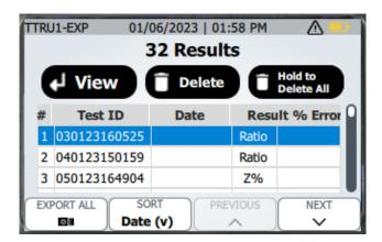
Test results are listed with a test number, Test ID, Date of test, Result type (Ratio, Go/No Go, or Z%), and % error. % error will be blank if primary or secondary information was not saved with the result. % error will be Pass or Fail if the result is a go/no go impedance test.
