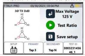
Press the enter key to select the maximum test voltage from the following options: 1 V, 4 V, 8V, 16 V, 32 V, 50 V, 80 V, 125 V, 160 V, 200 V, or 250 V. Voltages above 50 V will use the step up method of ratio testing.
