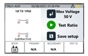
Clicking the SAVE button will save the vector, primary, and secondary winding information as a custom vector based on the TEST ID. Custom vector primary and secondary winding information can be updated and resaved to update the custom vector. Up to 10 custom vectors can be saved.
