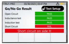
Open circuit ensures continuity through a winding.
