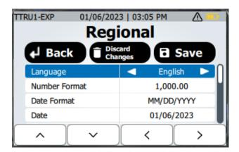
Press the back button to return to the settings screen without saving the changes
