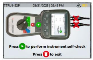
Follow the directions on screen to complete the device self check.
