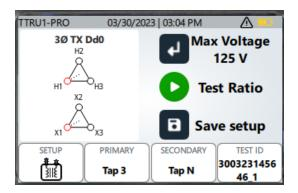
Press the enter key to select the maximum test voltage from the following options: 1 V, 4 V, 8V, 16 V, 32 V, 50 V, 80 V, or 125 V. Voltages above 50 V will use the step up method of ratio testing.
