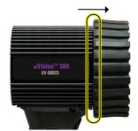
The Clear Borofloat Filter will remain inside the protector. To remove the Clear Borofloat Filter (130089), peel around the edge of the rubber cover/filter holder and push the filter out. To replace or reinsert the Clear Borofloat Filter into the rubber cover/filter holder, slide the Clear Borofloat Filter into the channel of the rubber cover/filter holder. Manipulate the rubber cover around the filter. Assure the filter is evenly seated.
