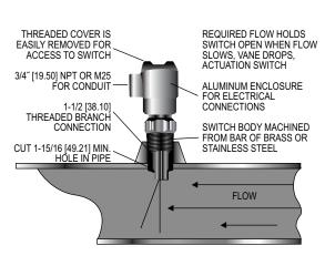
Threaded Branch Connection Installation. May also be installed using tee, flange or coupling.
