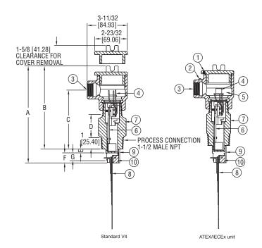
5. For units supplied with both internal ground and external bonding terminals, the ground screw inside the housing must be used to ground the control. The external bonding screw is for supplementary bonding when allowed or required by local code. When external bonding conductor is required, conductor must be wrapped a minimum of 180° about the external bonding screw. See below.
