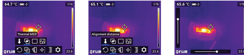
Figure 7.5 Select the Thermal MSX mode and then the Alignment Distance option. Use the sliders (left side and bottom of the display) to align the Digital Camera image with the Thermal image. Use the left/right and up/down arrow buttons to make the adjustments.
