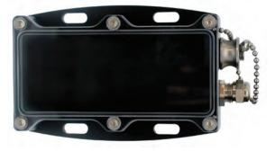
mounting holes for easy surface attachment. The enclosure features a water-tight communication access plug with chain attachment, stainless steel probe outlet and a clear plastic cover.
